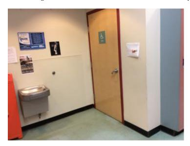
PM7 - Door handles were found to be broken on most boy's and girl's restrooms. We recommend replacing the broken handles and keeping all restroom doors open during school hours.
